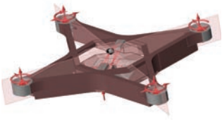
Initial Design Space with loading applied in Inspire
