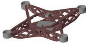
Inspire Optimization on the Airframe conditions
